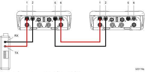
Figure 2 Connecting multiple DCM or ADCM.
